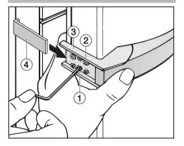
■ First, loosely screw the door handle onto the opposite side, using the two forward screws ②.
